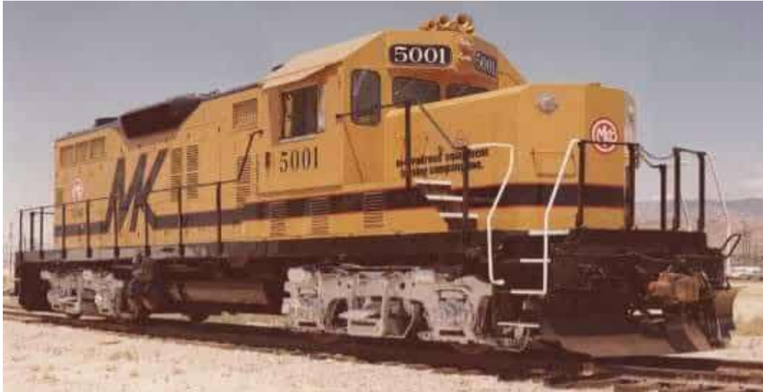
M&K Leasing Locomotive Nr. 5001, with one Sulzer 6ASL25 in Service between 1979 and ~2006 (Foto DG 80)
