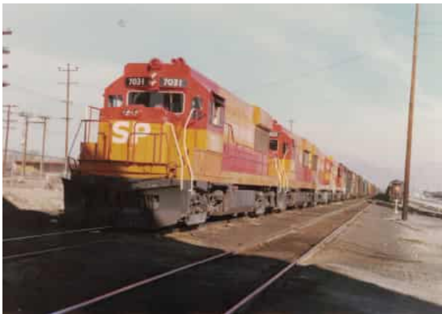
Southern Pacific Locomotives Nr. 7030-7034, each with one Sulzer 12ASV25 of 3'240 BHP operating about 140'000 US miles from 1978-1980 (Foto DG 80).
